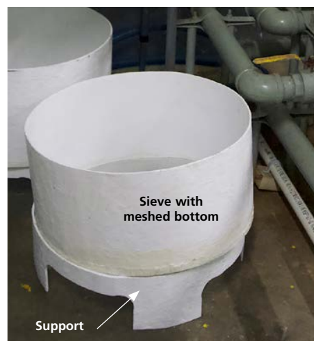
Fiberglass sieve with independent support
