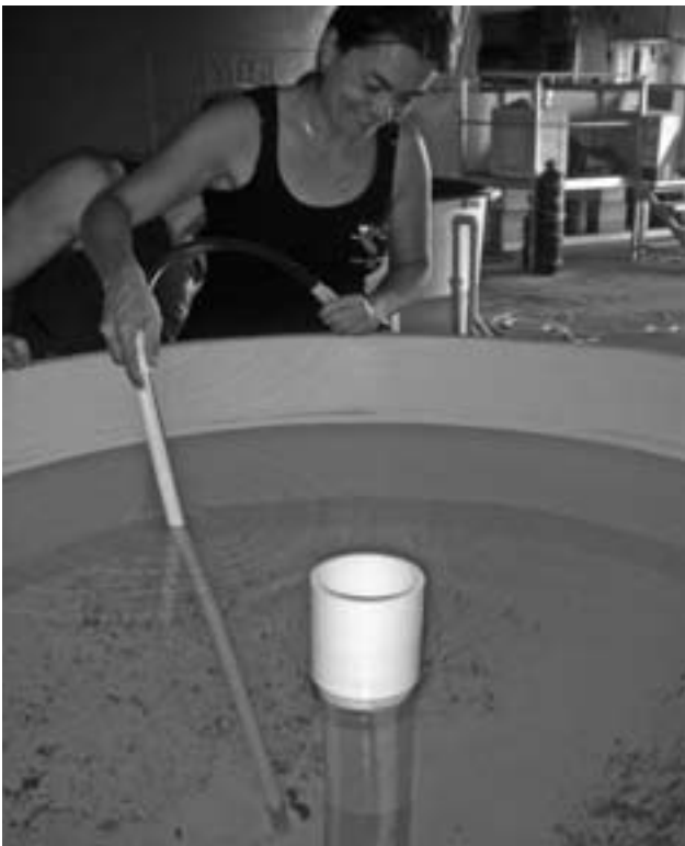
Figure 42. Detachment by siphoning.
