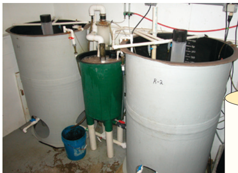
Figure 2: Recirculating rotifer production system.
