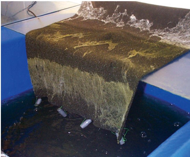
Figure 3: Typical batch culture tank with floc trap pulled out of tank.
