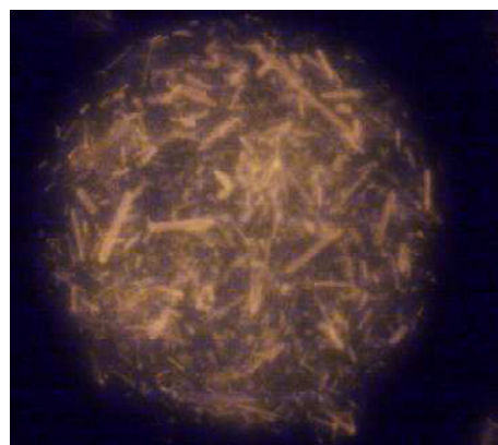
Fig. 7. LSB prepared with paraffin wax, soy lecithin and cod liver oil ( 227 \text{ g kg}^{-1} , 545 \text{ g kg}^{-1} and 164 \text{ g kg}^{-1} ) and 64 \text{ g kg}^{-1} riboflavin (Table 3, LSB type 1). The picture was taken using an epifluorescent microscope (Leica DM1000, Leica inc) fitted with a UV light source (excitation of 450–490 nm and emission of 515–528 nm). LSB were dispersed in seawater for 1 h and 55 min and riboflavin particles were still visible within the beads.
