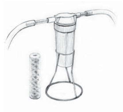
Fig. 8. Bio-filter (with bio-filter cartridge shown separately)
