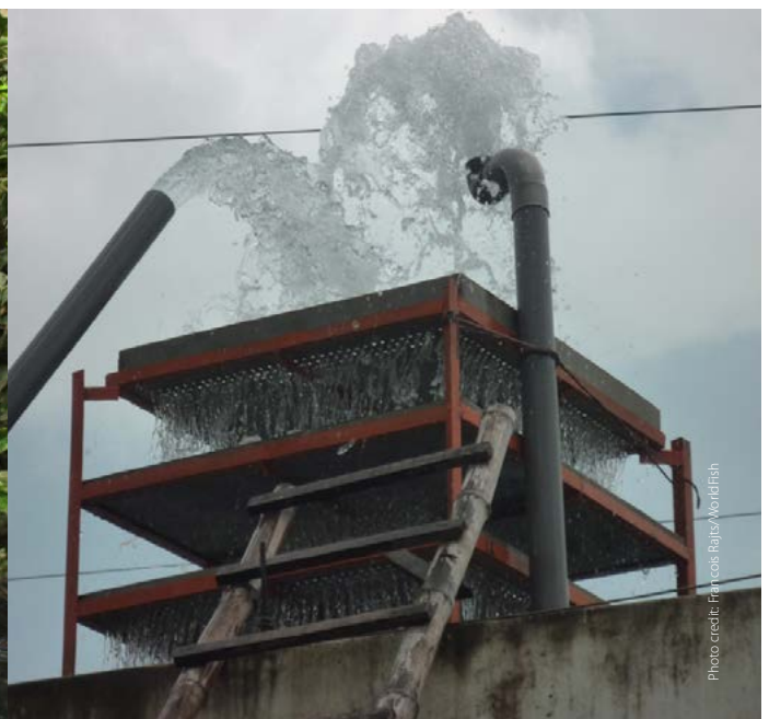
Plate 2. Aeration tower in a small hatchery in Sierra Leone (left) and an aeration tower (designed by F. Rajts) for a large hatchery in Bangladesh with high levels of carbon dioxide (right).
