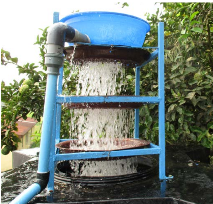
Plate 2. Aeration tower in a small hatchery in Sierra Leone (left) and an aeration tower (designed by F. Rajts) for a large hatchery in Bangladesh with high levels of carbon dioxide (right).
